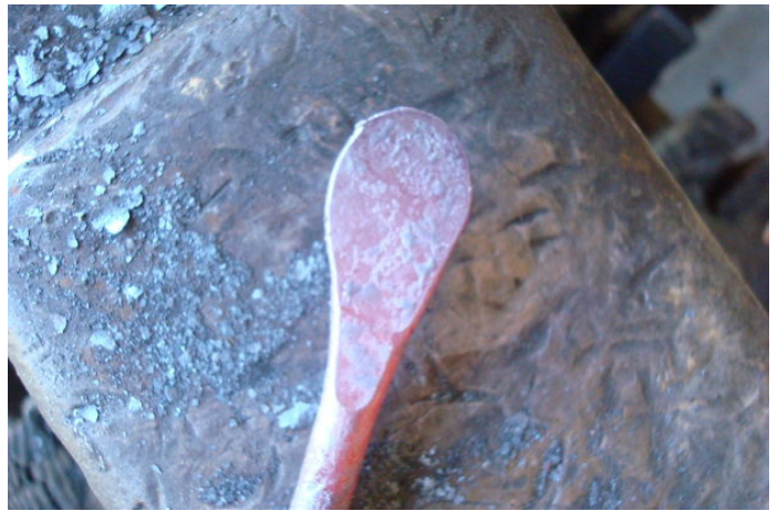
After bending J and cutting to length, flatten end.
