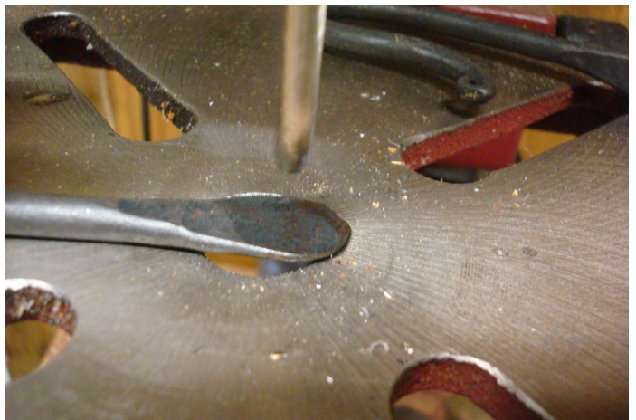
Drill a mounting hole using the drill press.
