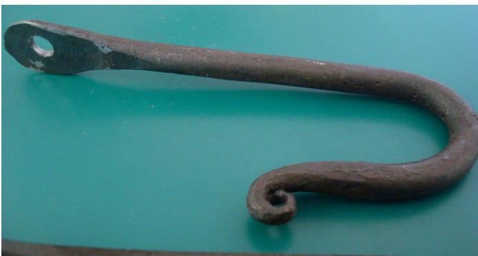
A completed “J” hook.
